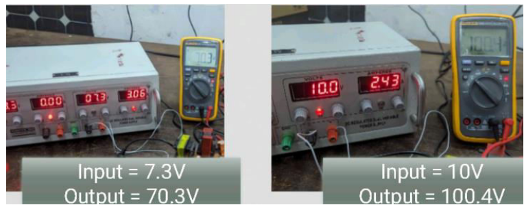
Fig. 11 Hardware output showing 10 times boosting of two different input voltages
